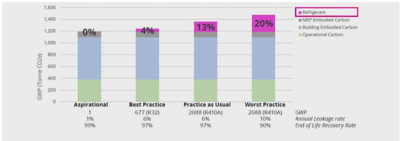
**Figure 4.14:** Whole life carbon emissions over 30 years of a US low energy office building (2,000 m<sup>2</sup>) using a VRF system. Depending on the refrigerant used, its leakage rate and recovery at end of life, refrigerant can have a different impact on global warming. (Source: Hamot et al., 2020).
